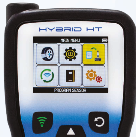
Select PROGRAM SENSOR on the main menu
