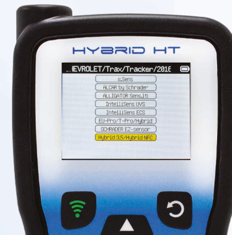
Choose the correct EU-Pro sensor generation
