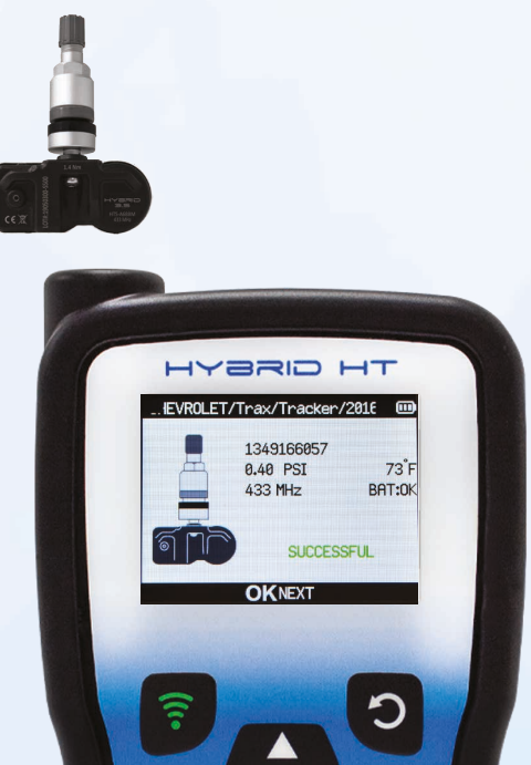
The tool will display SUCCESSFUL if the process was a success
