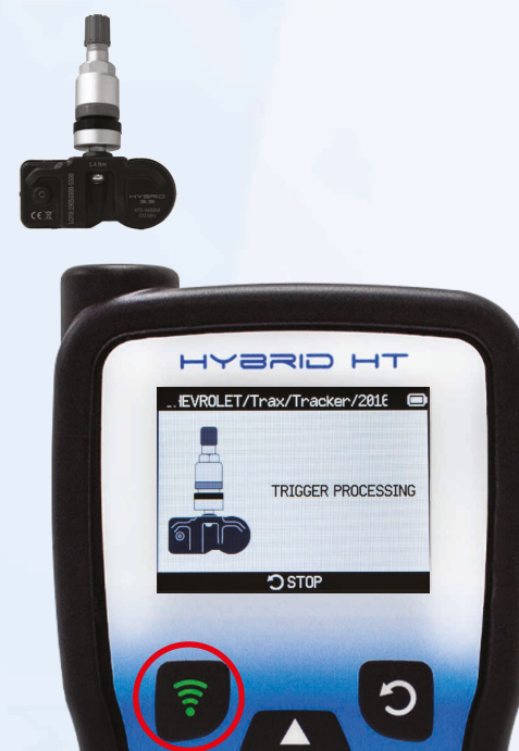
Press the green trigger button
